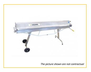
Lightweight manual construction site bending machine
