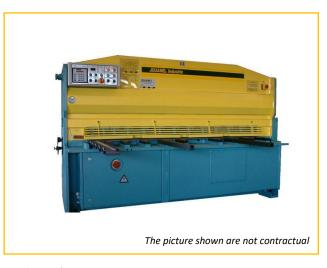
Hydraulic guillotine shear 4m x 6 mm
