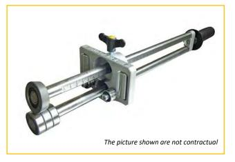
The folding roller inclined at 10°, specifically designed for bending without marking the material, will also make it possible to compensate for the spring back of the metal and thus obtain a true 90° fold.
